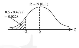
:. The percentage of rejected steel cables  $= 0.0228 \times 100 = 2.28\%$
